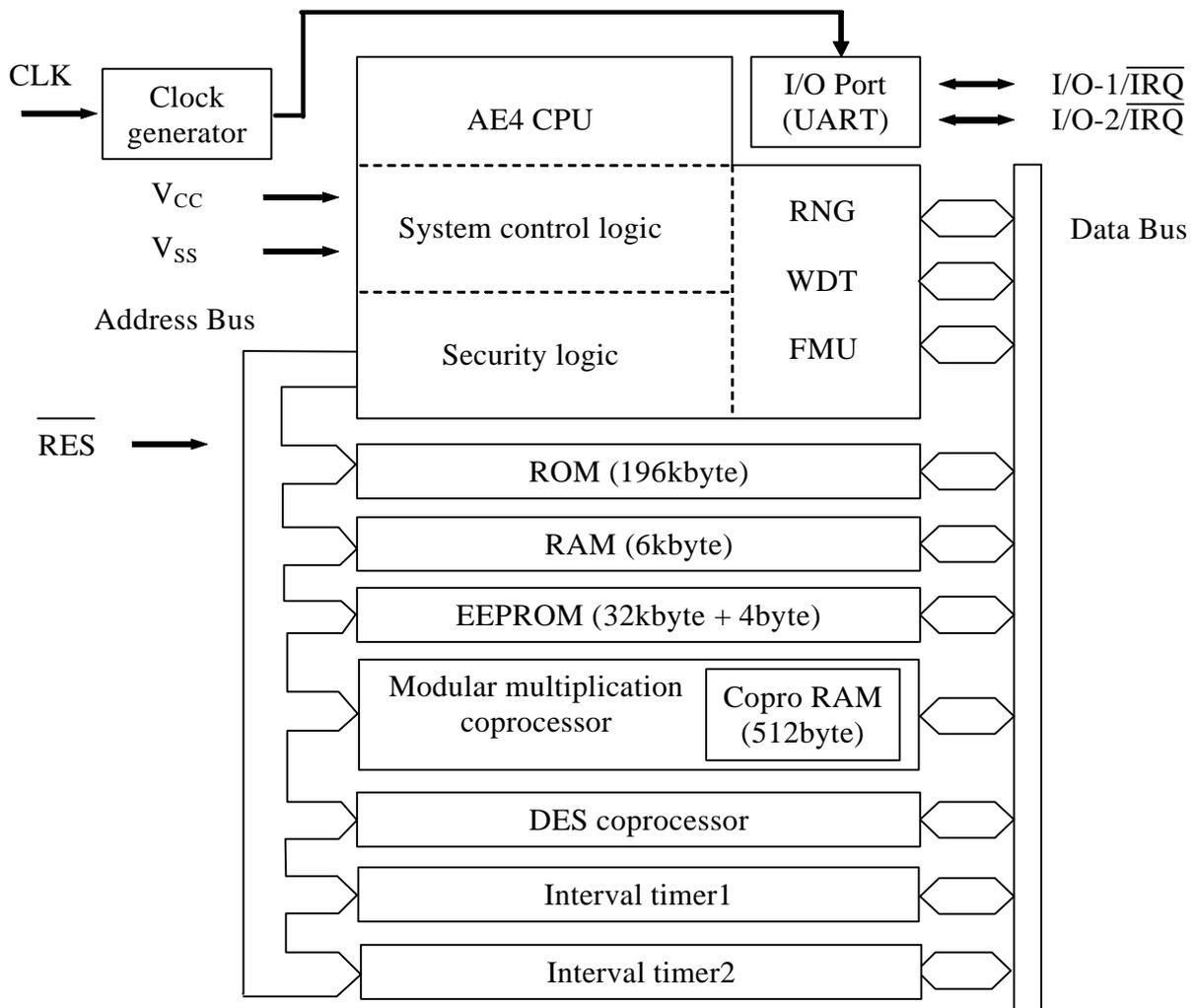
Figure 1: Internal block diagram of the AE45C1
