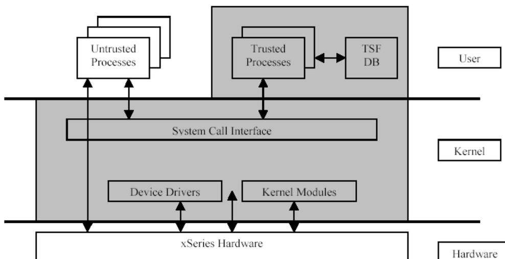
The kernel itself is structured into a number of subsystems which are explained in detail in the high level design of the TOE. Those are:
