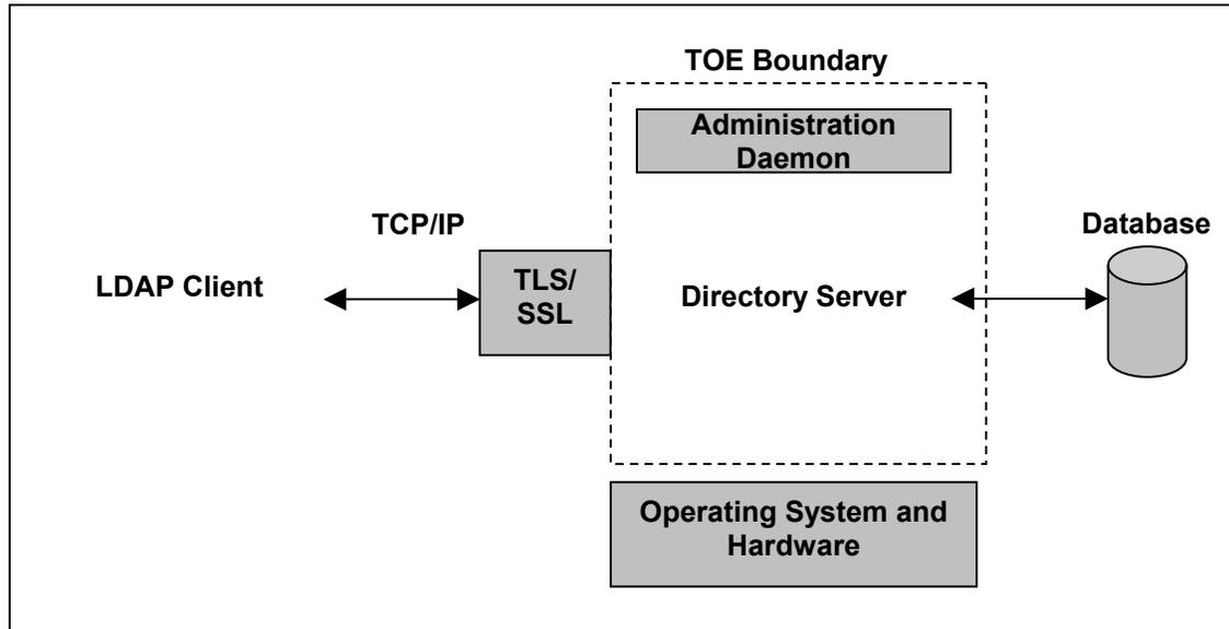
**Figure 1: IBM Tivoli Directory Architecture and TOE Boundary**
