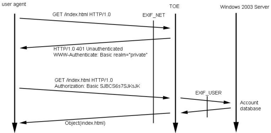
**Figure 6.2 – Web Identification & Authentication Process (Radius server)**
