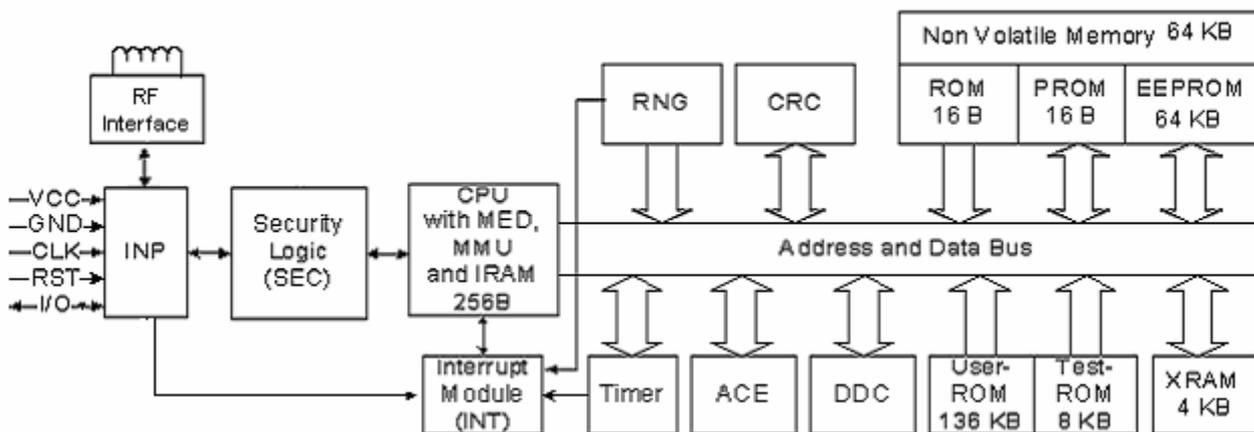
Figure 1: Block diagram of the SLE66CLX640P and SLE66CLX641P
