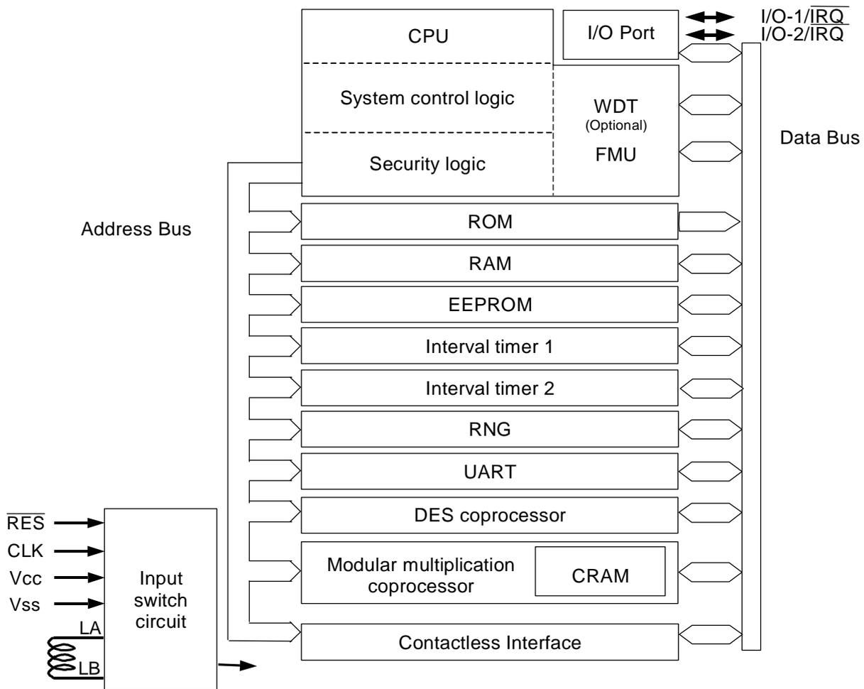
Figure 2-1: Internal Block Diagram of the TOE
