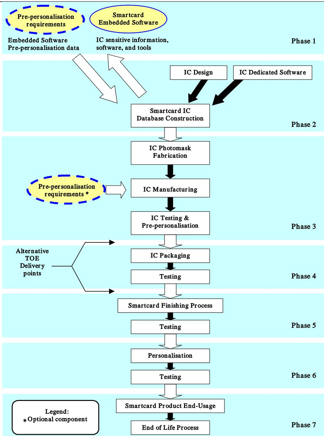
Figure 2-2: Design and Manufacturing Lifecycle
