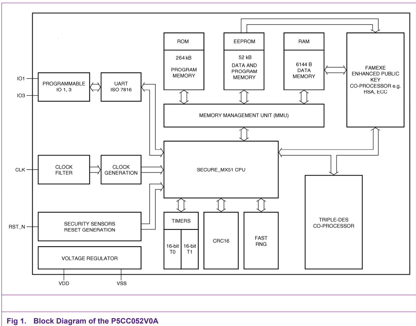
Fig 1. Block Diagram of the P5CC052V0A
