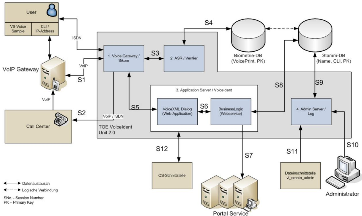
Figure 3: Voicident Unit 2.0 voice verification system
