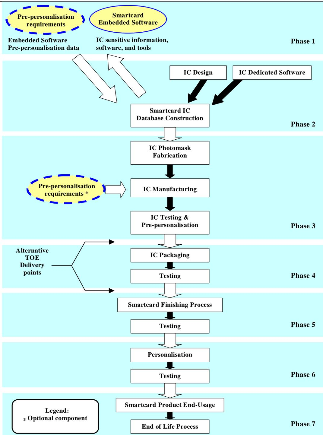
**Figure 2-2: Design and Manufacturing Lifecycle**
