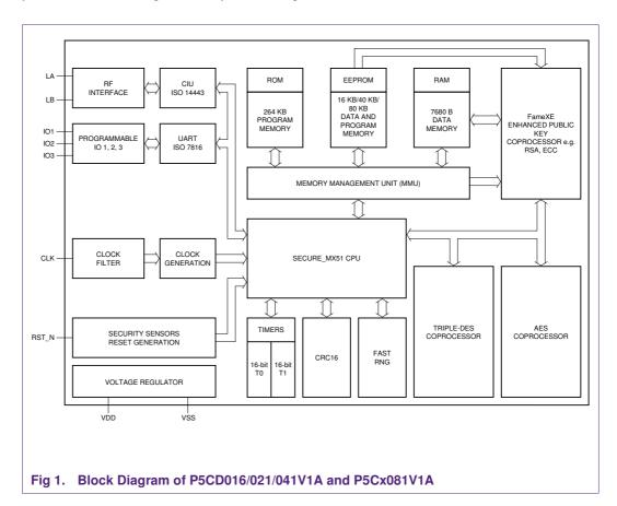
The TOE consists of the IC hardware and the IC Dedicated Software as composed of IC Dedicated Test Software and IC Dedicated Support Software. All other software is called Security IC Embedded Software and is not part of the TOE. The following table lists the TOE components.
