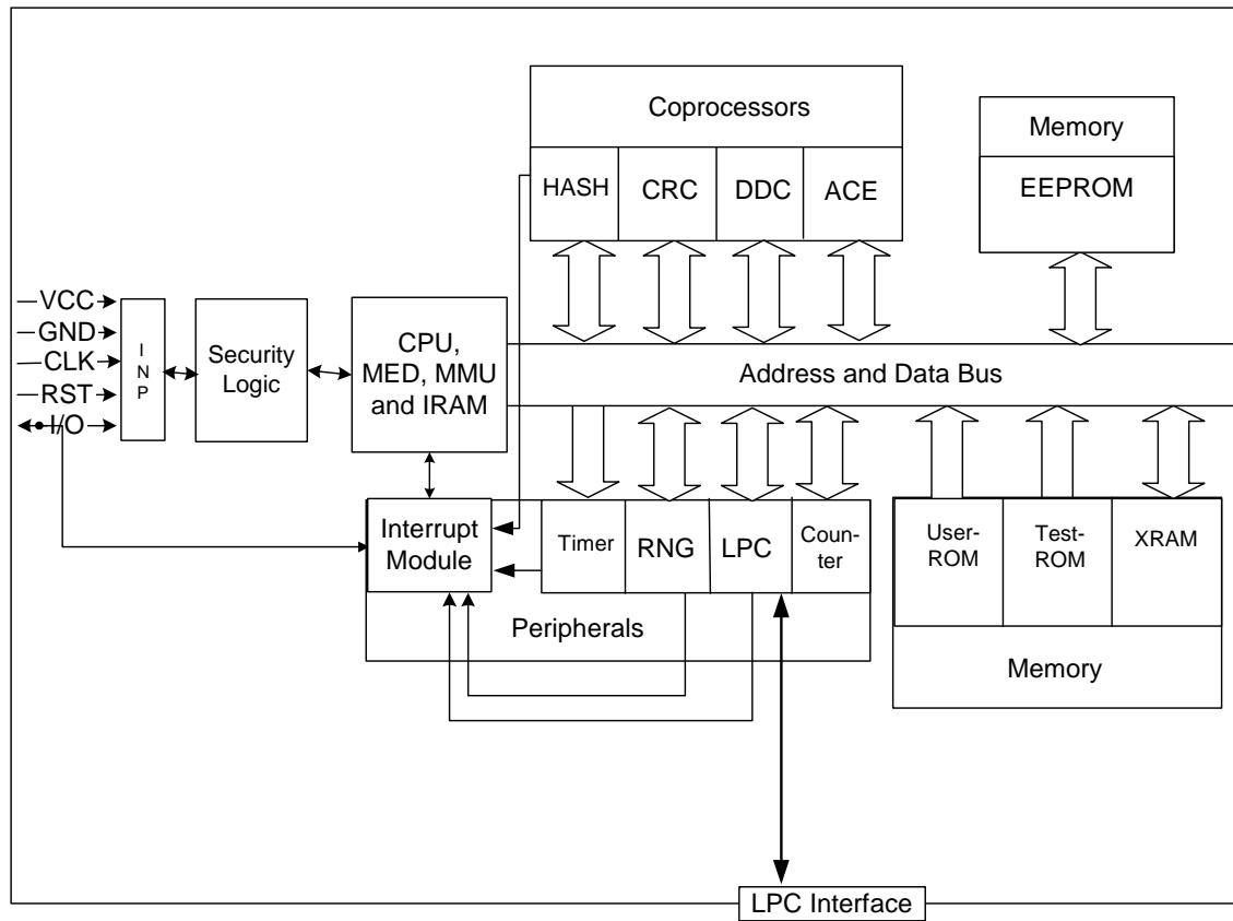
Figure 1: Block diagram of the SLB9635TT1.2
