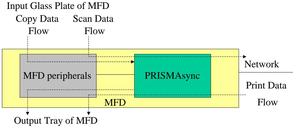
**Figure 1: Relation between the Océ PRISMAsync and MFD.**
