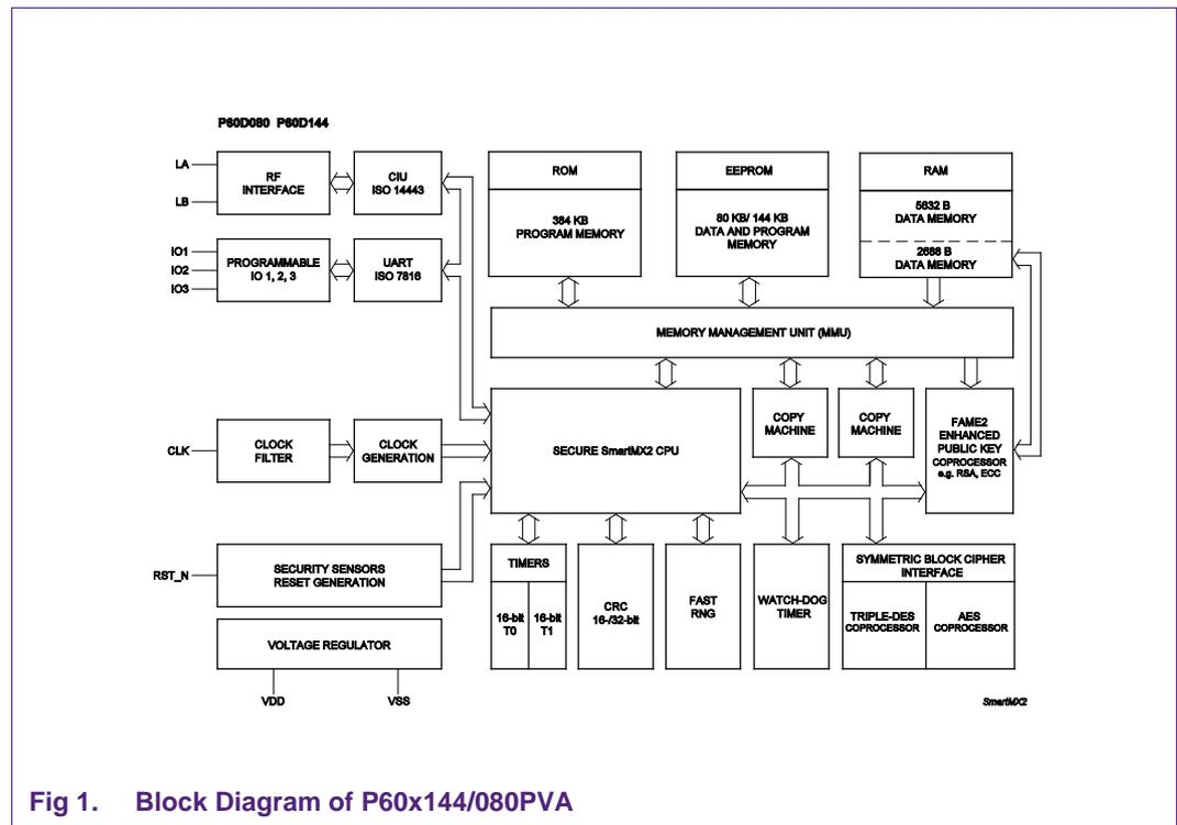
Fig 1. Block Diagram of P60x144/080PVA
