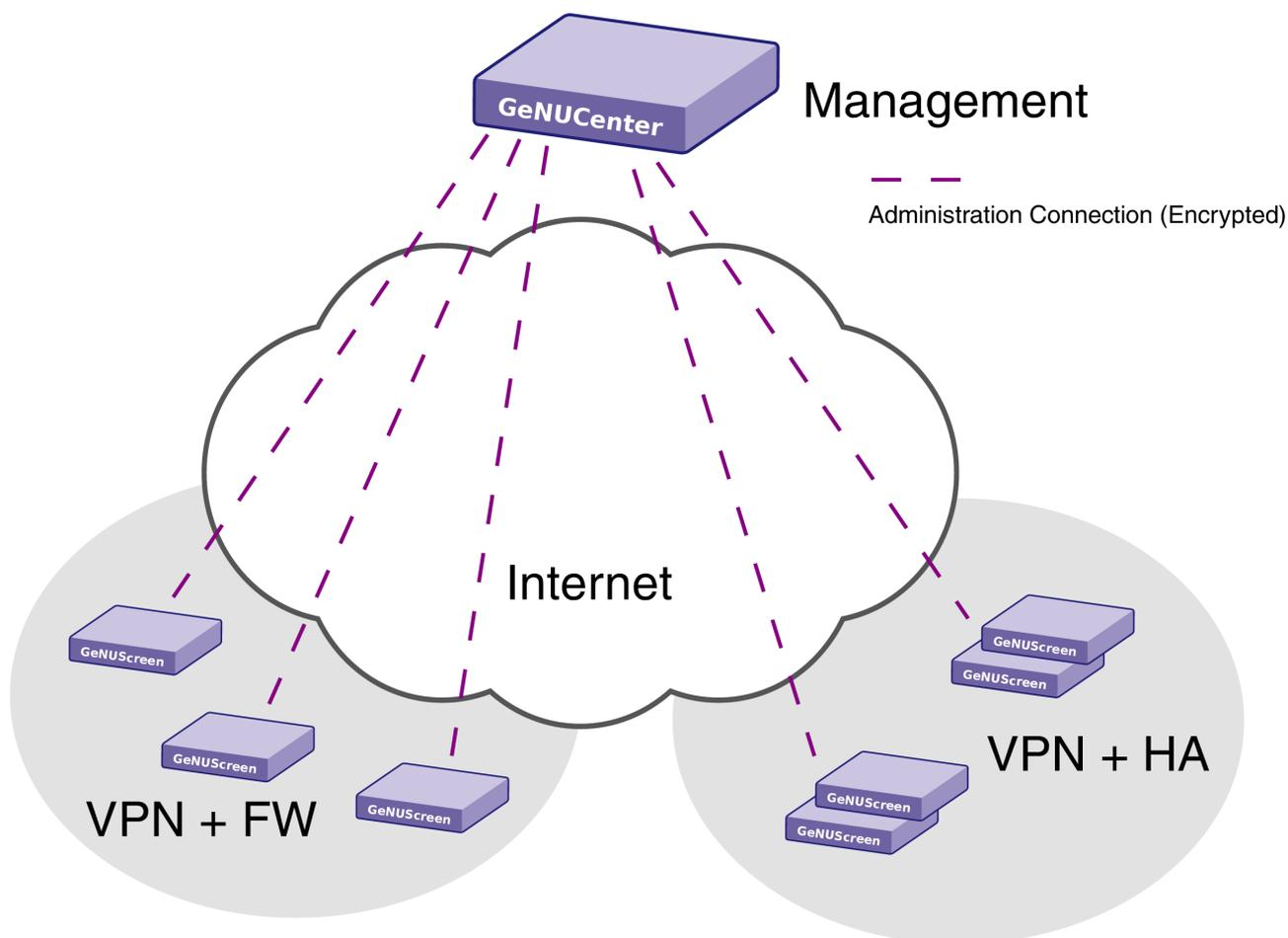
Figure 1: Two genuscreen virtual private networks managed by genucenter. The VPN on the left has additional packet filter rules for unencrypted communication. The VPN on the right is using the HA option.
