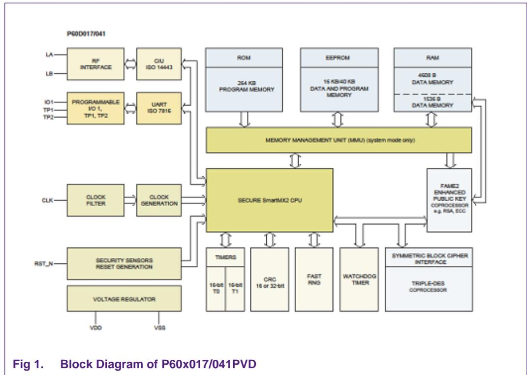
Fig 1. Block Diagram of P60x017/041PVD
