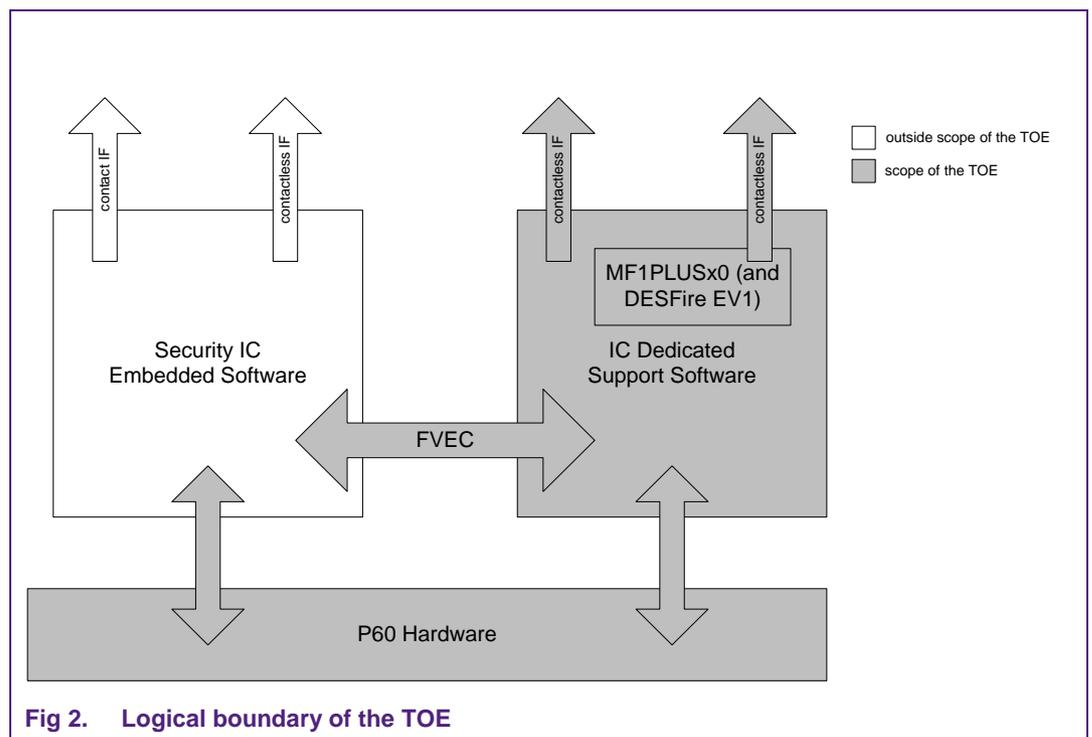
Fig 2. Logical boundary of the TOE
