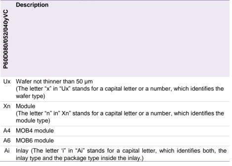
For example, commercial type name P60D080MX0/9Crrff2 denotes major configuration P60D080MVC with MIFARE Plus MF1PLUSx0 supporting 2 kBytes of EEPROM and PDM1.1 dual interface smart card module. The characters 'rr' and 'ff' are individual for each customer product.
