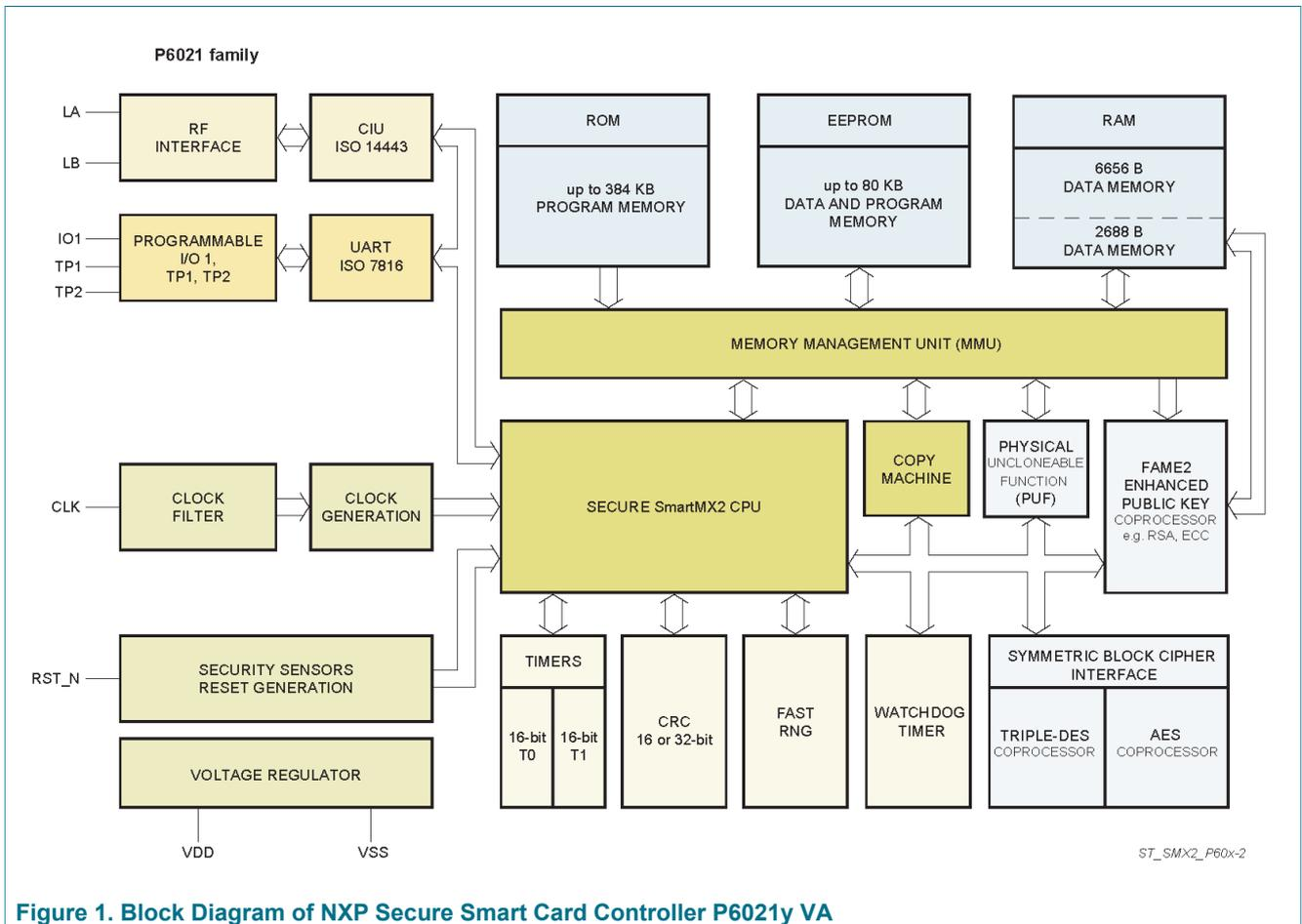
**Figure 1. Block Diagram of NXP Secure Smart Card Controller P6021y VA**
