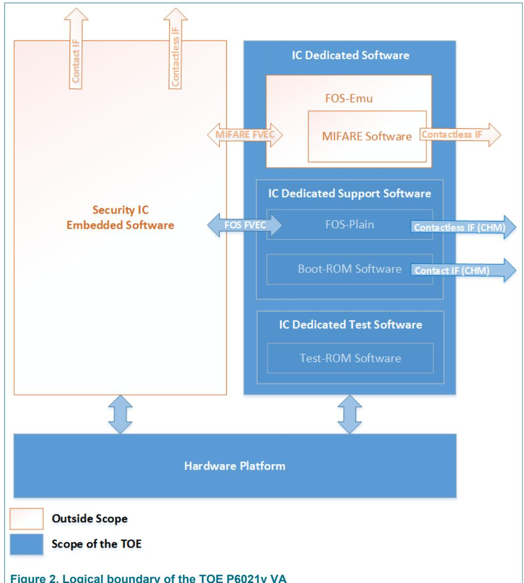
Figure 2. Logical boundary of the TOE P6021y VA
