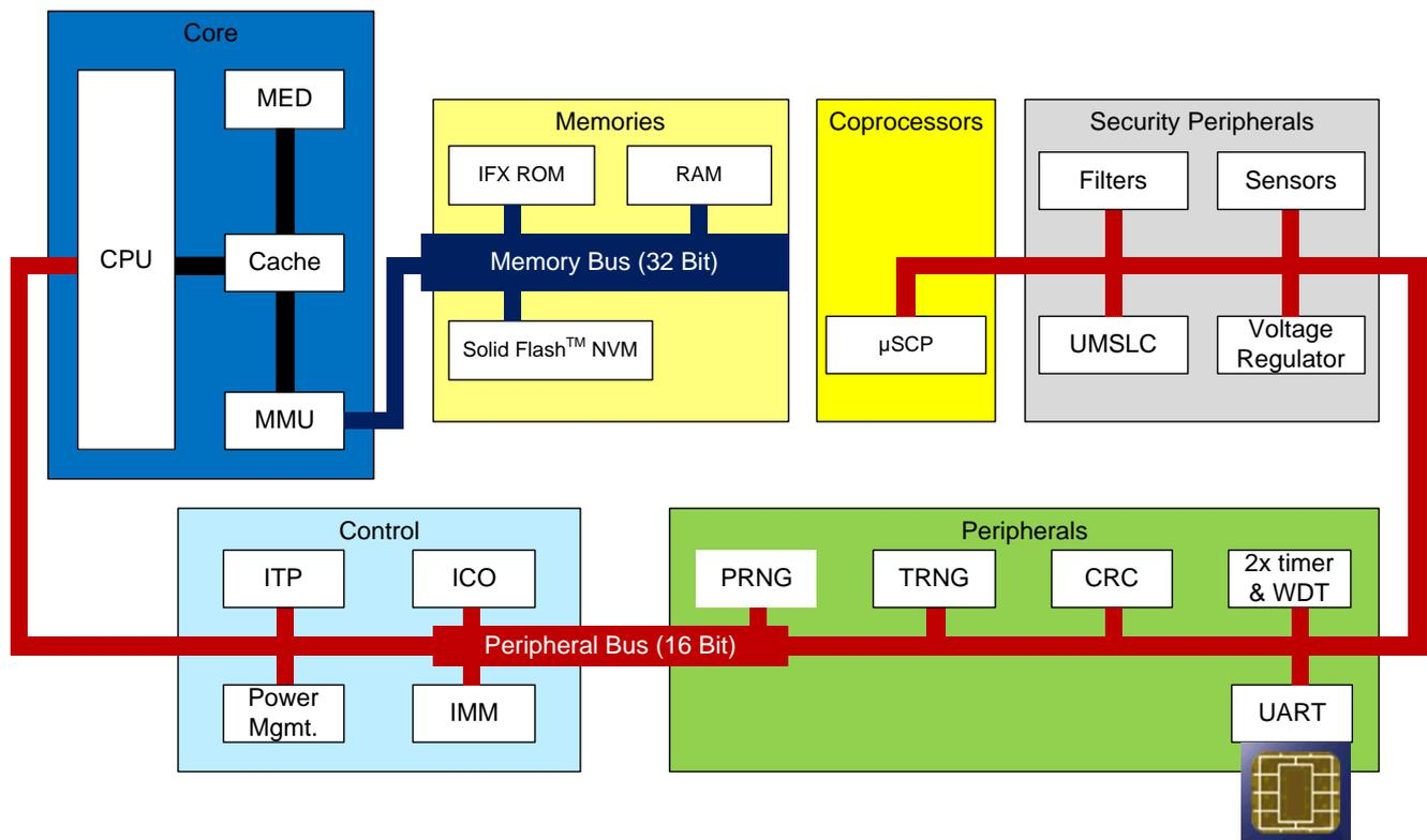
The TOE consists of a core system, memories, coprocessor, peripherals, security modules and control peripherals.
