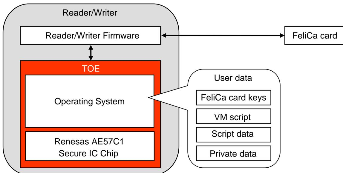
**Figure 1: Functional configuration of the reader/writer and the TOE**
