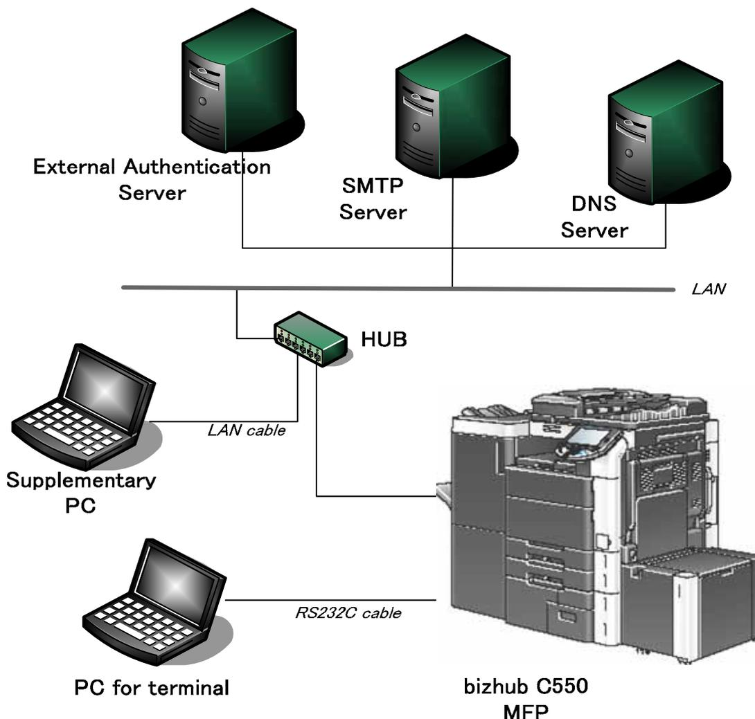
**Figure 2-1 Configuration of Developer Testing**
