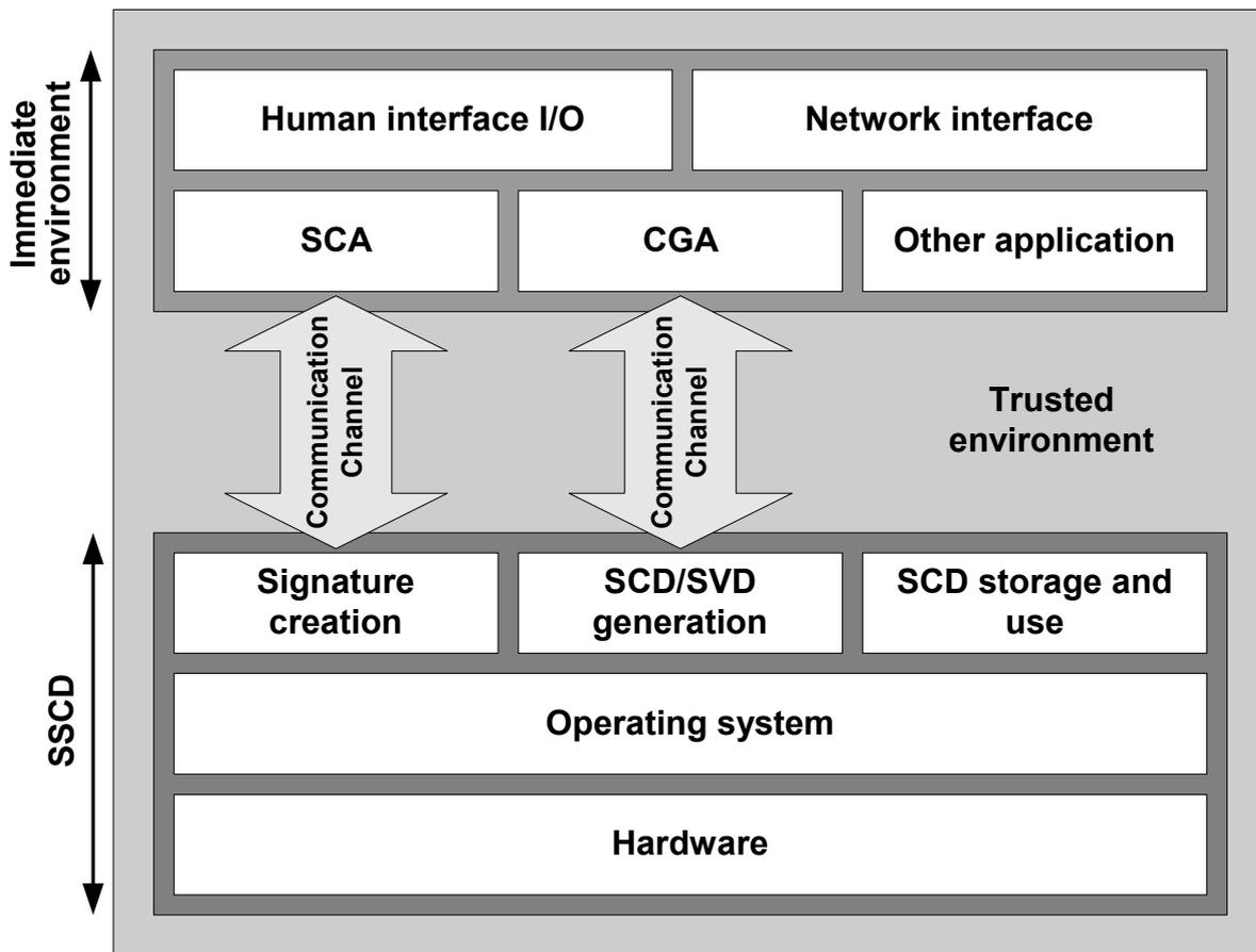
**Figure 1: Scope of the SSCD, structural view**
