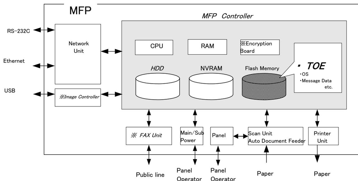
**Figure 2 Hardware composition that relates to TOE**
