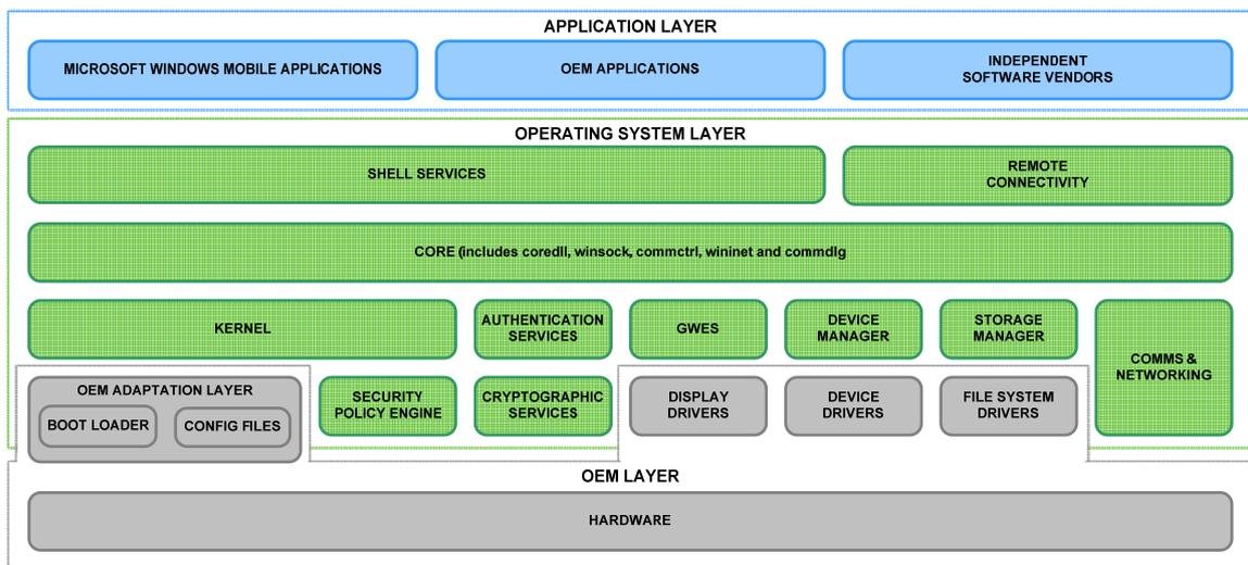
Figure 2: TOE Architecture
