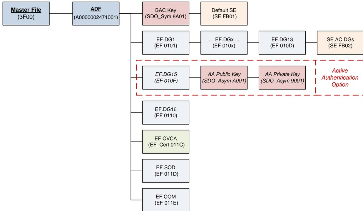
Figure 2 - Typical BAC LDS for IDPass
