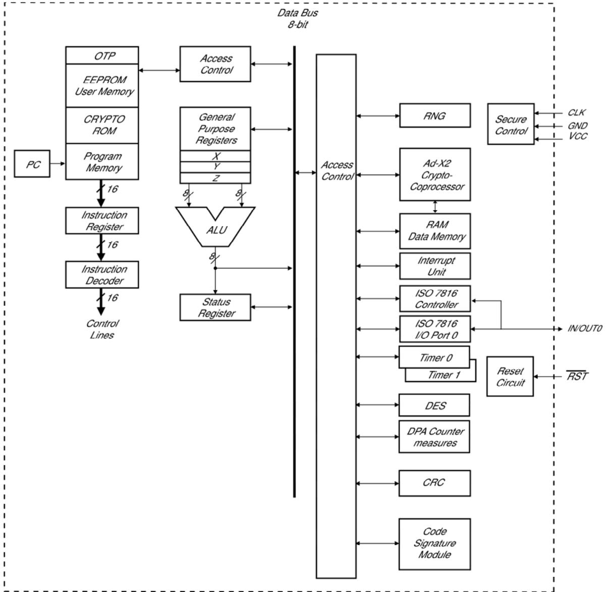
Figure 1: Block Diagram of the AT90SC24036RCV TOE
