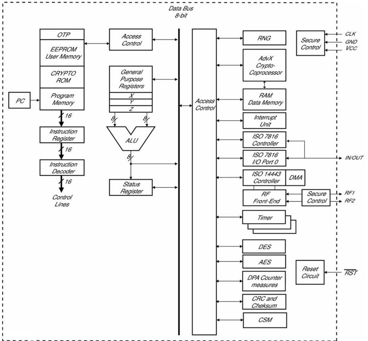
Figure 1: Block Diagram of the AT90SC28880RCFV TOE
