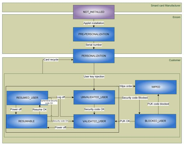
Figure 2: Cryptosmart card life cycle
