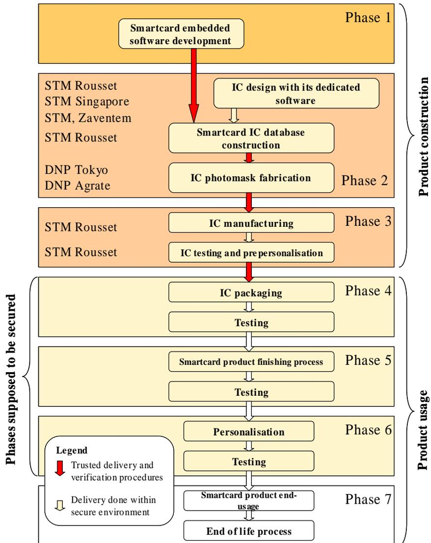
Figure 1 – Life cycle of a smart card
