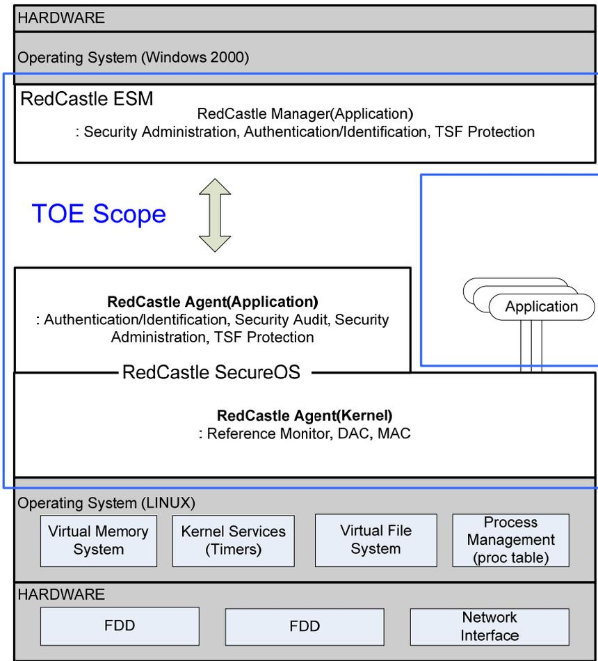
[Figure 2-2] Physical TOE Scope
