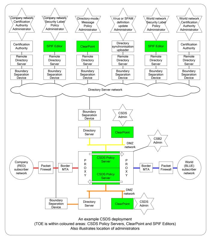
This is just a single example of one of the many permitted configurations of a deployed TOE.
