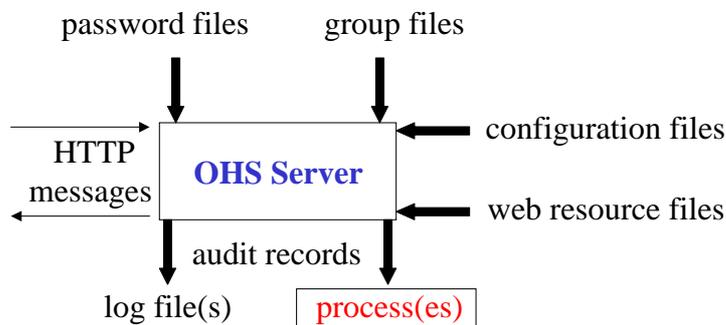
57. The figure below illustrates input/output for the htpasswd program, which is the part of the TOE that performs security attribute management. Disk access is achieved via the operating system.
