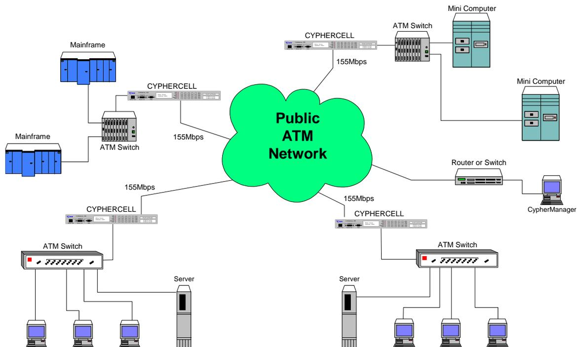
Figure 3 – A Secure ATM Network
