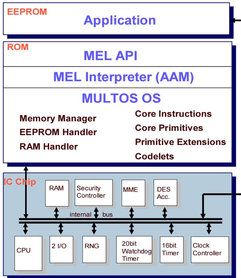
TOE is implemented in the IC chip which is Samsung Electronics's S3CC9RB or S3CC9P9 certified CC EAL4+. The IC chip contains CPU that performs commands including executable code of MULTOS. Also it contains hardware for implementing the function of cryptography.
