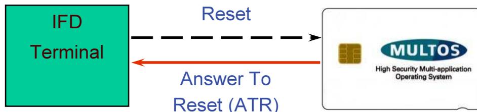
An MCD (MULTOS Carrier Device) sends ATR(Answer-to-Reset) to an IFD when receiving Reset signal from the IFD. After that half-duplex communication starts between the IFD and MULTOS with command-response pairs, where a command is a message from the IFD to MCD and a response is a message from MCD to the IFD.
