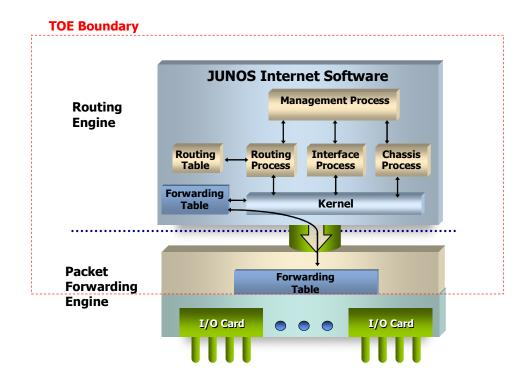
The interfaces to the TOE are twofold: the routing interfaces and the management interfaces. The management interfaces include the TOE console interface through which the router can be managed locally and the in-band management interface via the
