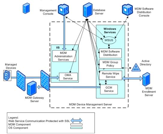
Figure 6 – Components of the MDM Device Management Server
