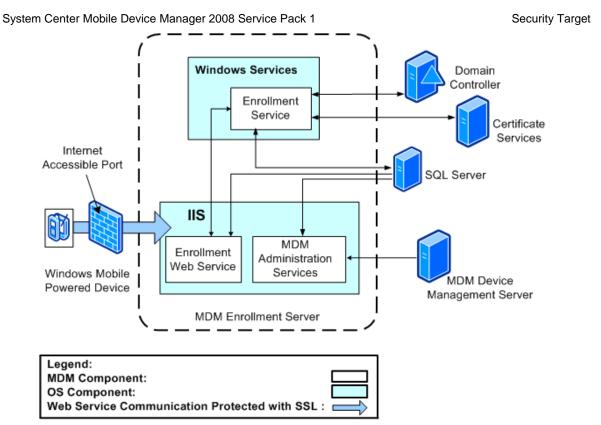
Figure 5 – Components of the MDM Enrollment Server
