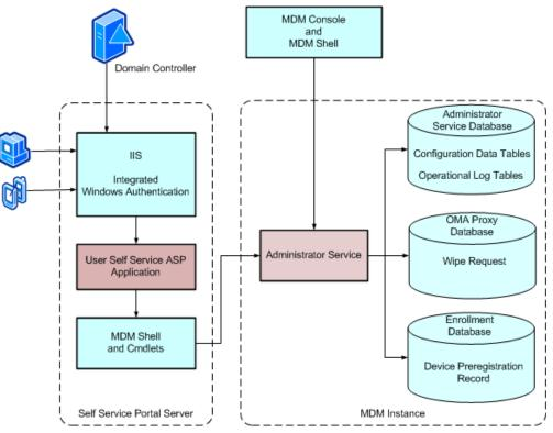
Figure 7 – Components of the MDM Self Service Portal
