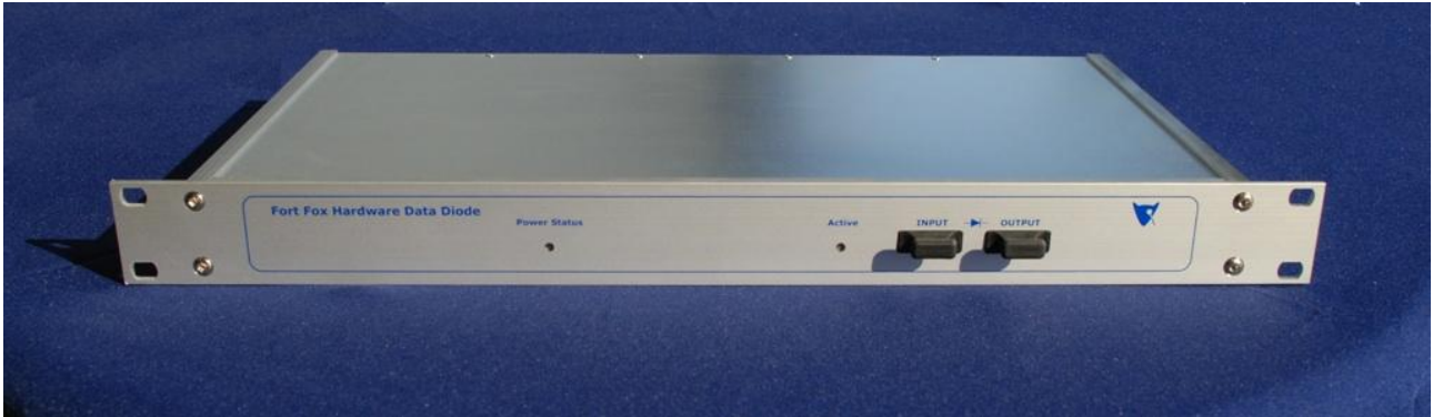
Figure 2: The TOE as a single 19" rack component
