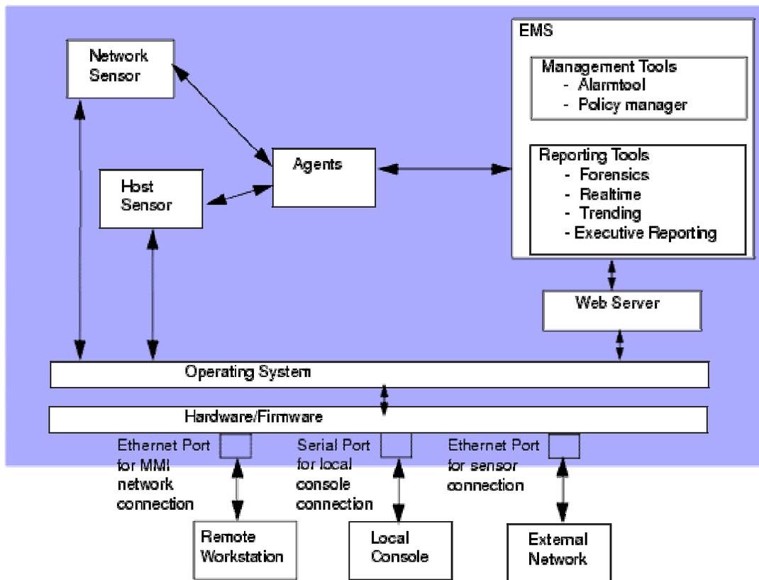
Figure 2: Dragon-EAL™ Component Architecture
