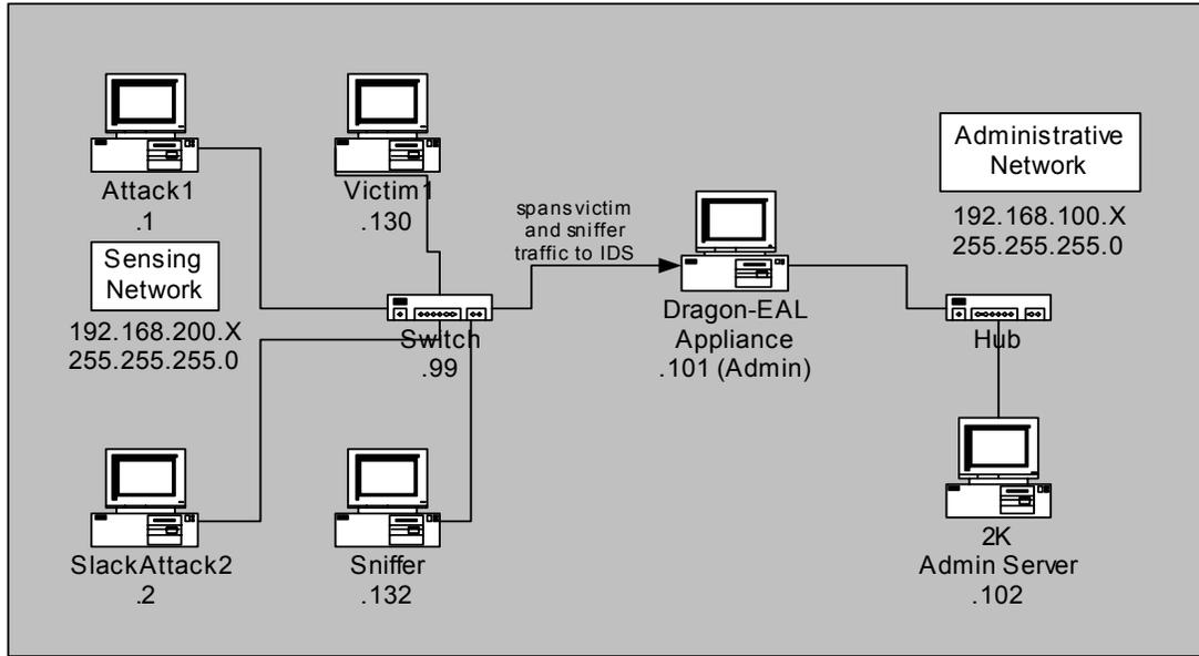
Figure 3: Enterasys Dragon-EAL testing environment
