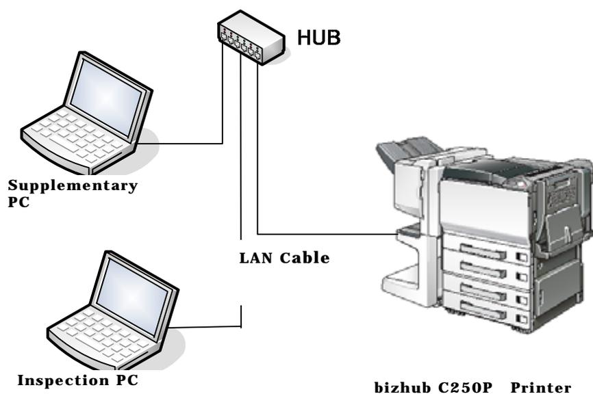
Figure2-2 Developer test ( Intrusion test ) configuration
