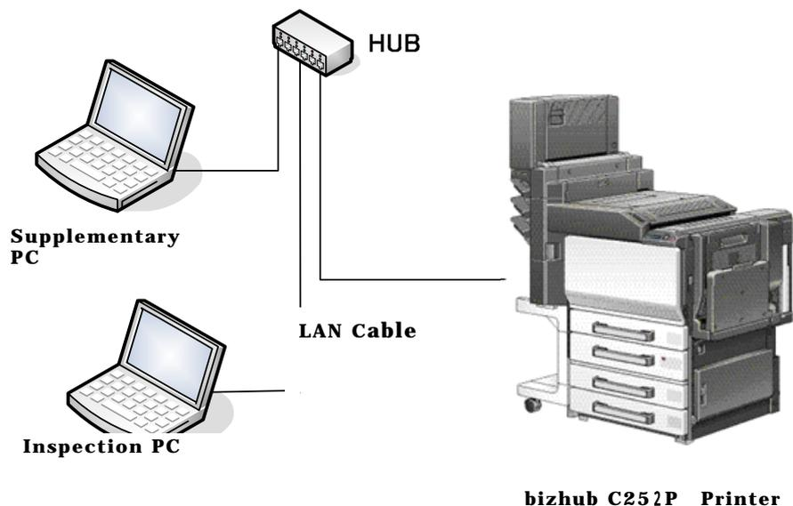
Figure0-2 Developer test ( Intrusion test ) configuration
