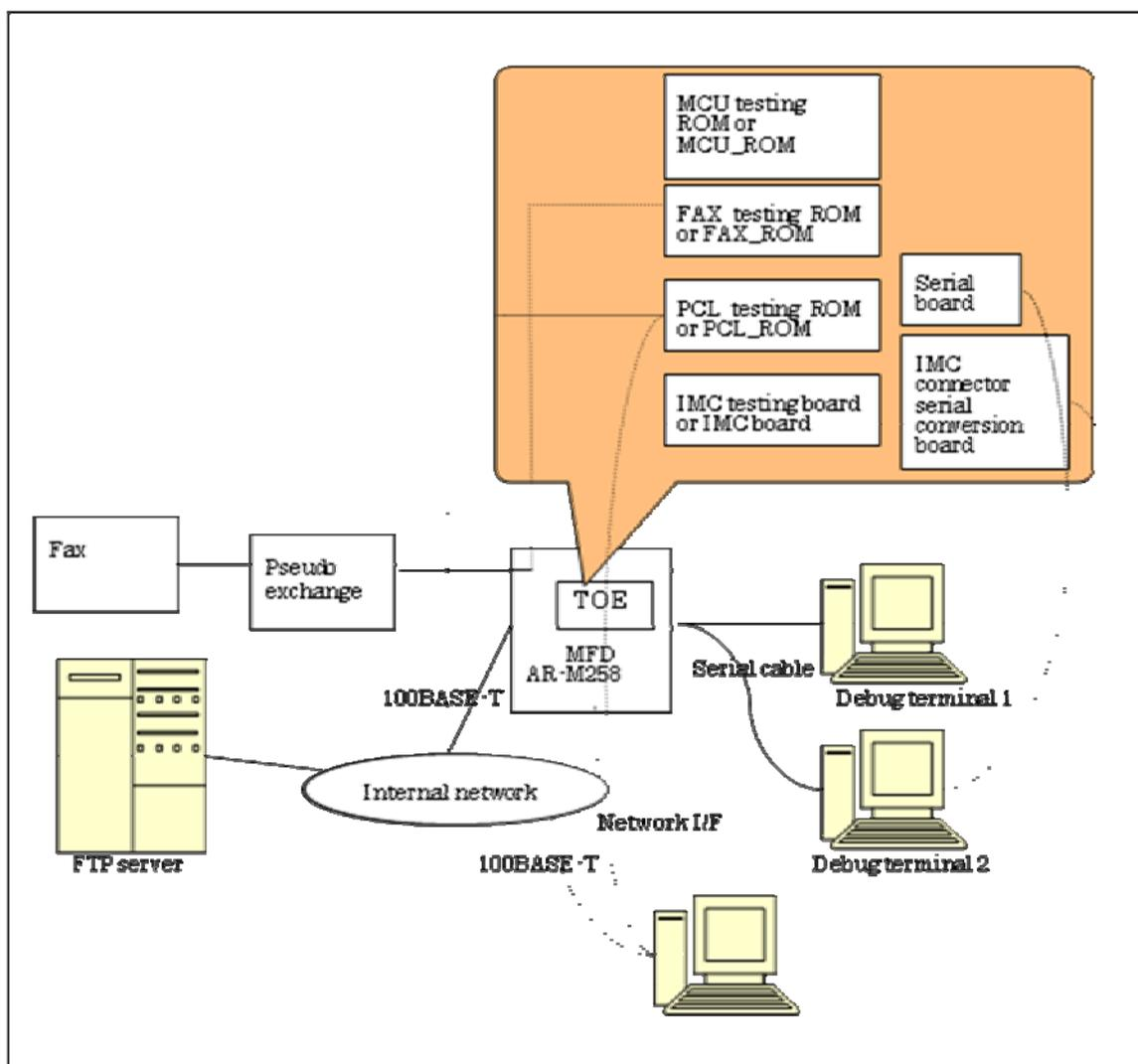
Figure 2-1: Configuration of Developer Testing
