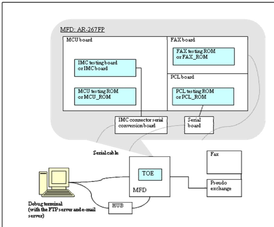
Figure 2-2: Configuration of Independent Testing
