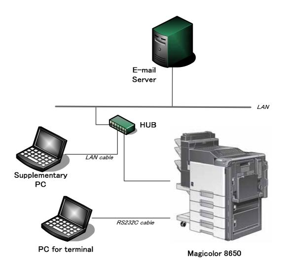
Figure 2-1 Configuration of Developer Testing
