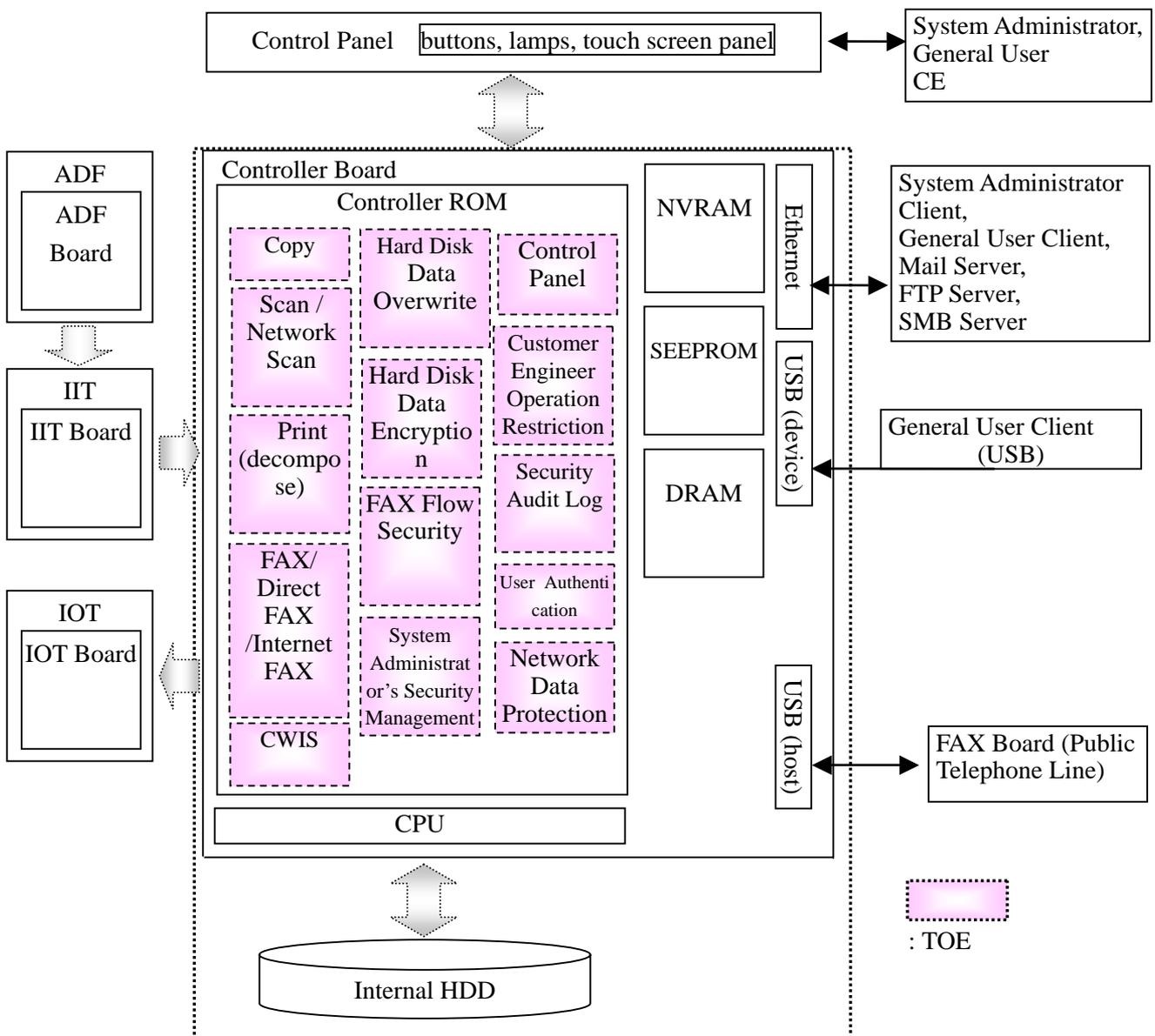
Figure 4: MFP Units and TOE Physical Scope
