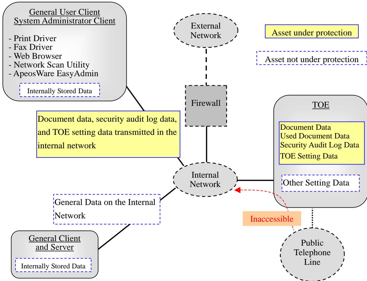
Figure 5: Assets under and not under Protection
