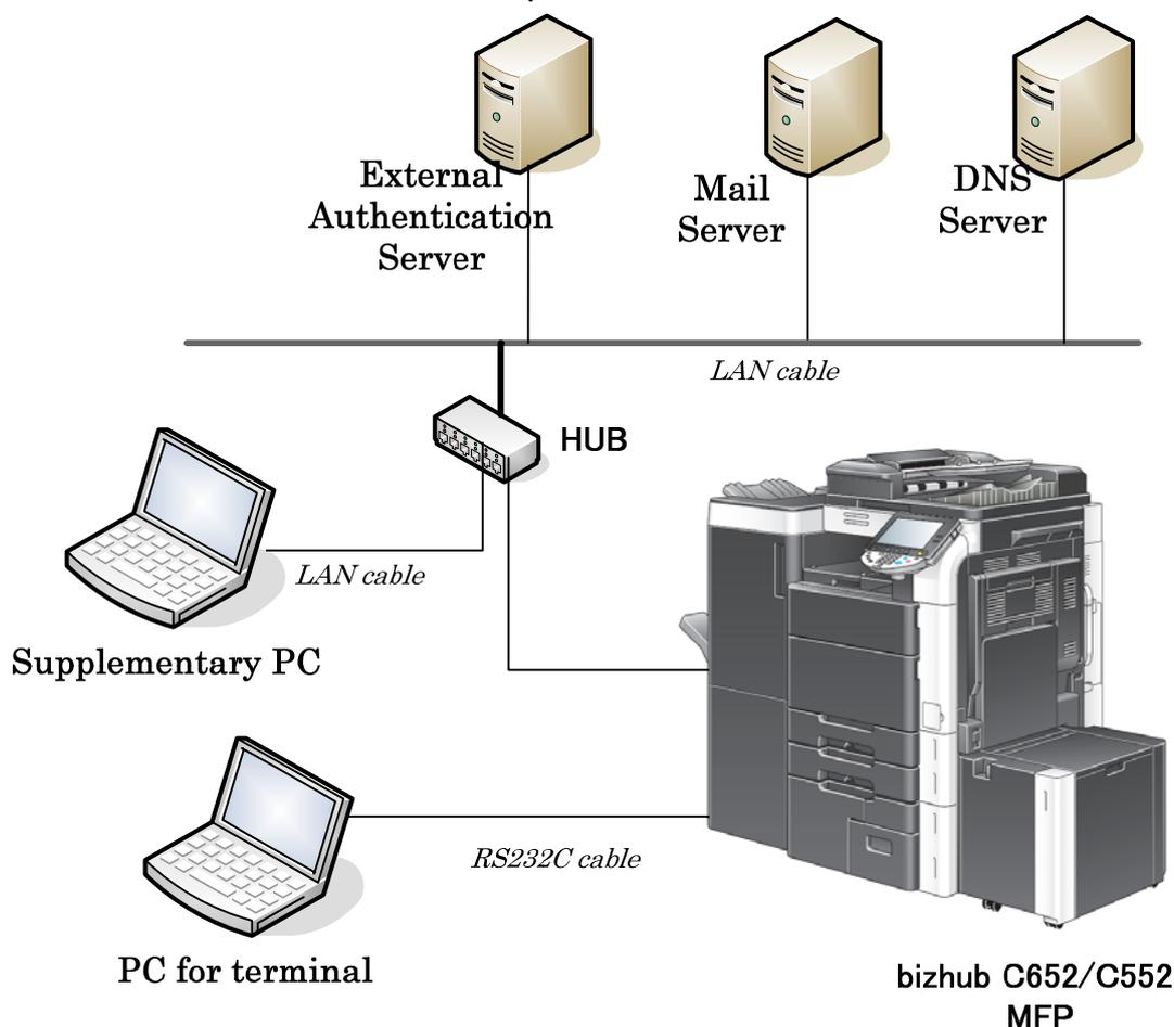
**Figure 3-1 Configuration of Developer Testing**
