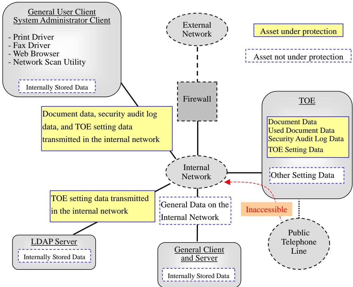
Figure 5: Assets under and not under Protection
