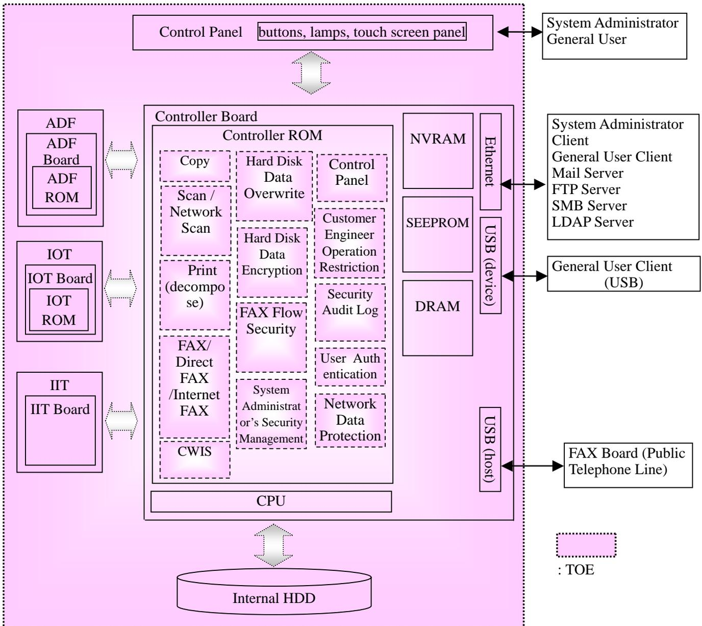
Figure 4: MFD Units and TOE Physical Scope
