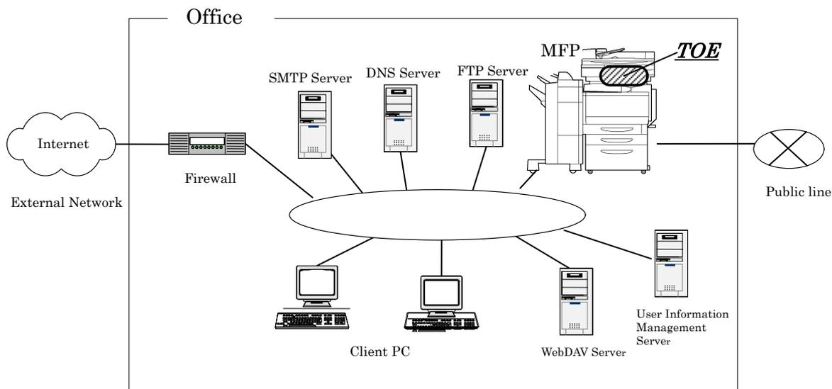
**Figure 1 An example of MFP's use environments**
