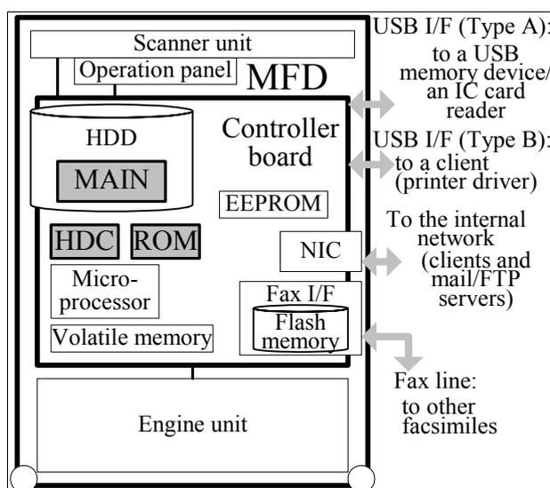
Figure 2: TOE and physical configuration of the MFD
