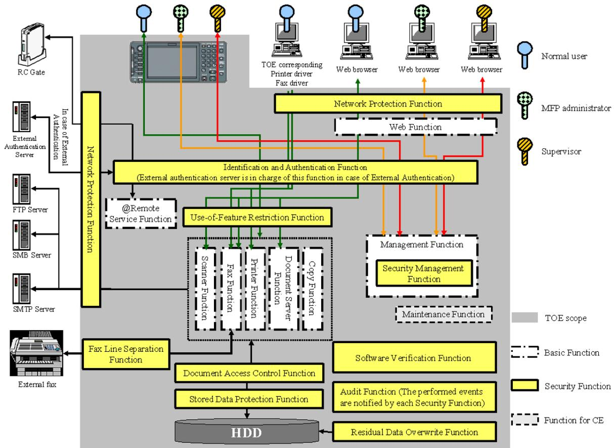
Figure 3 : Logical Scope of the TOE
