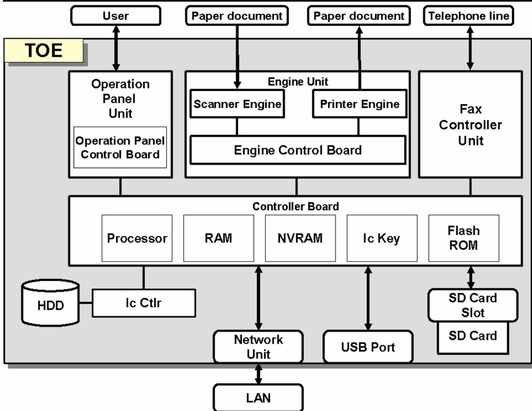
Figure 2 : Hardware Configuration of the TOE
