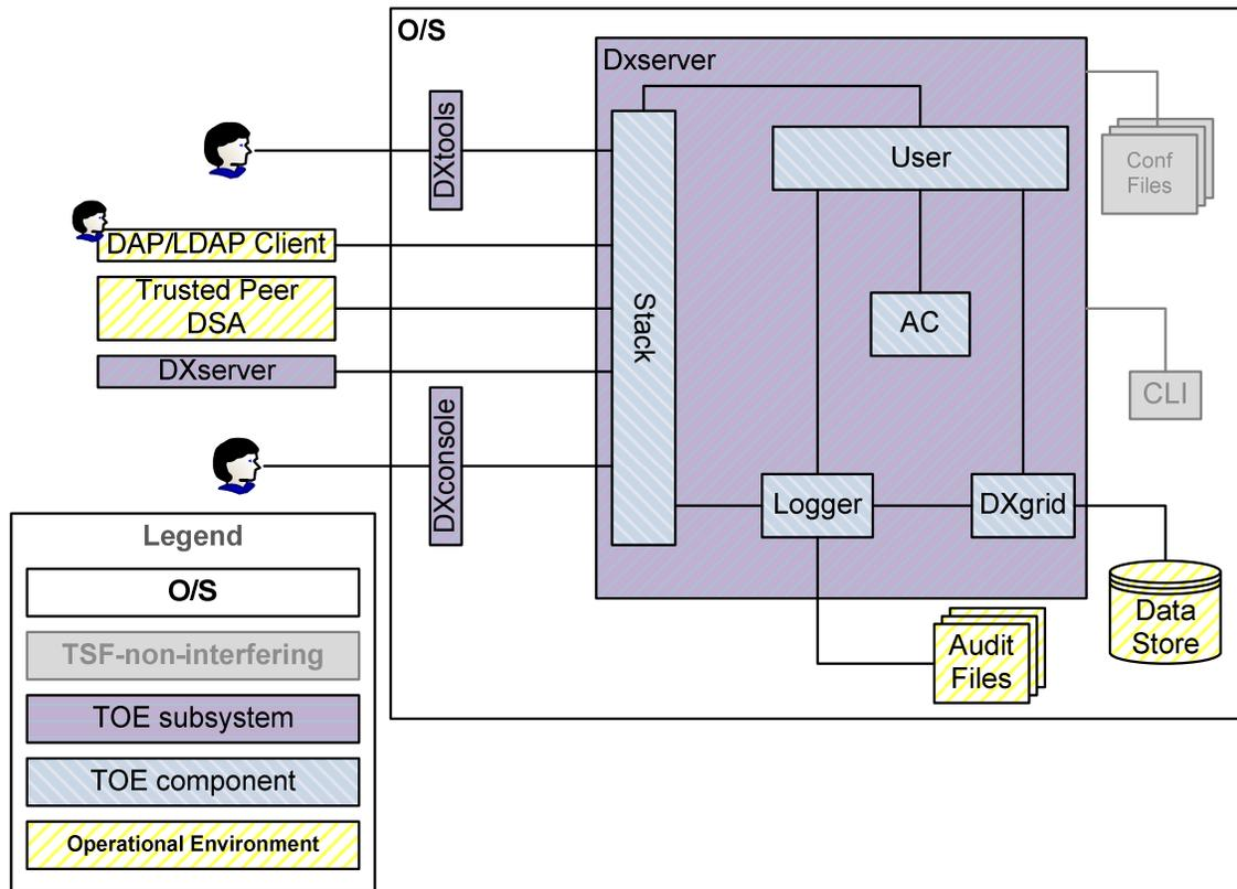
Figure 1 – TOE Boundary as Data DSA
