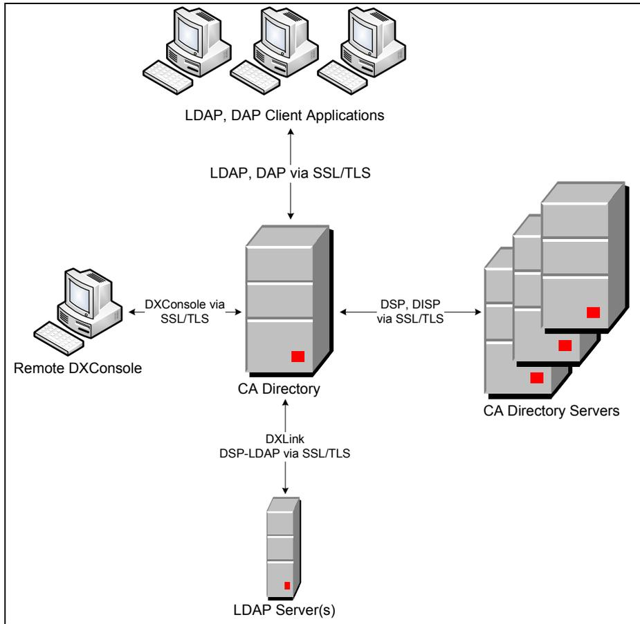
**Figure 3 – TOE Deployment**
